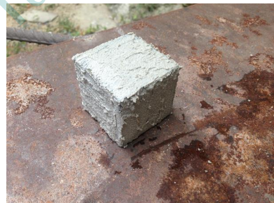
Figure 3 Coated specimens with epoxy
