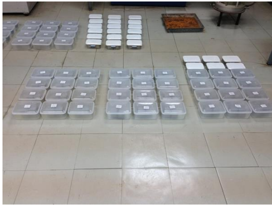
Figure 4 Immersing specimens in 3% sodium chloride box
