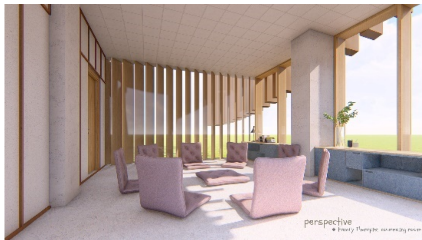
Figure 9 Landscape of group counseling for the families of women with unintended pregnancy 1, showing the amount of light brought into the building via clerestories and laths which are the sunshades of the building
