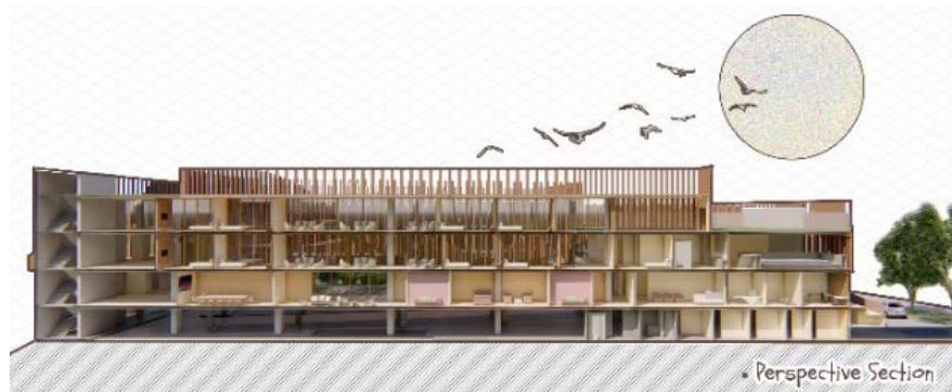
Figure 8 Section 2 shows the amount of natural light brought into the building through open spaces and clerestories of the building
