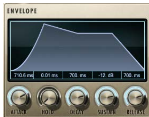
Figure 5 The adjusted sound envelope of the tremolo
