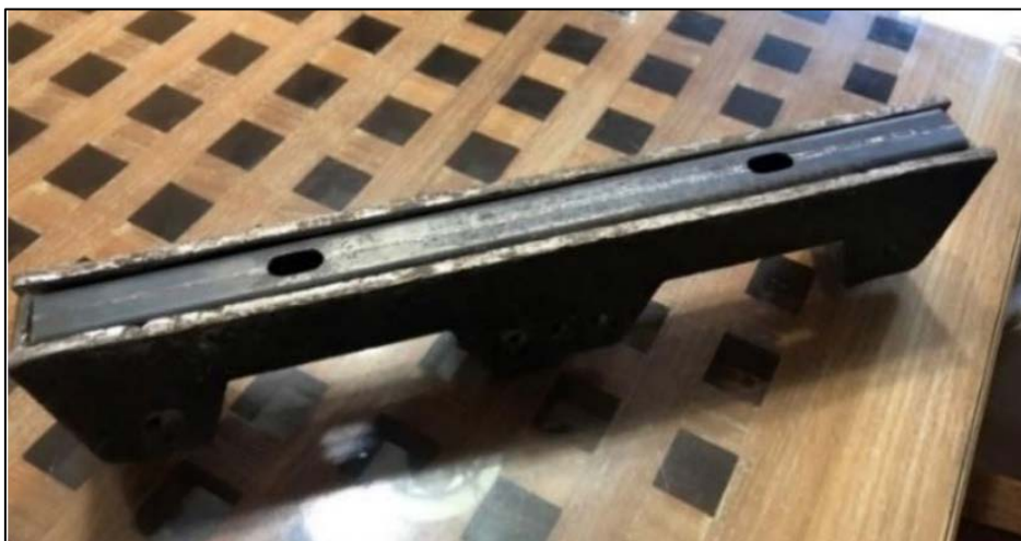
Figure 4 An example of the design of a mortar box lid from a flat steel
