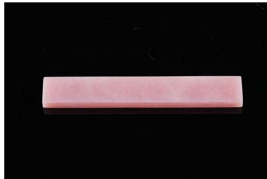
Figure 1 Polished silane-treated 10 weight % aluminum oxide (particle size 50-70 \mu\text{m} .) reinforced heat-polymerized acrylic resin specimen (size 65*10*3 mm 3 )
