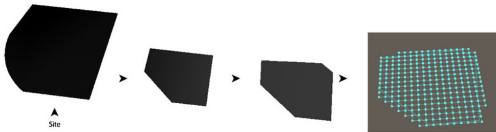
Figure 7 Site analysis as a way to find original mesh for form-finding process
