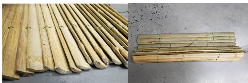
Figure 9 Bamboo chopped overlap (left) and bamboo roll (right)
