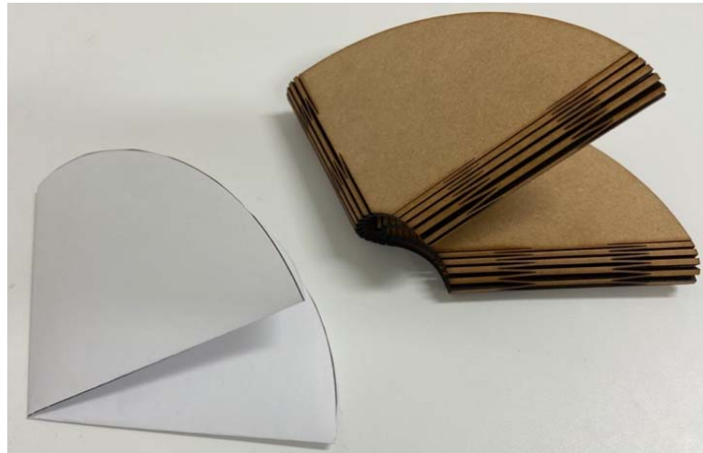
Figure 6 Folding model with lattice hinge
