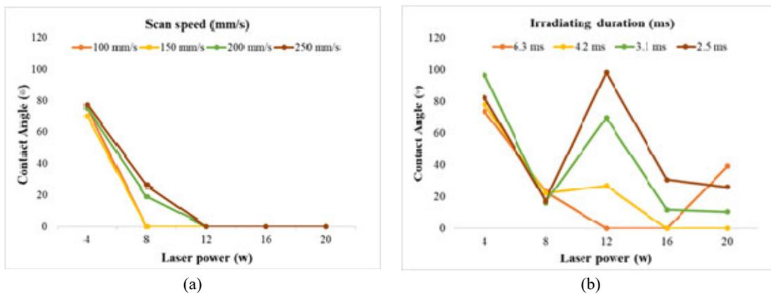
**Figure 5** Effect of laser power and scan speed on contact angle when texturing the (a) line and (b) point patterns
