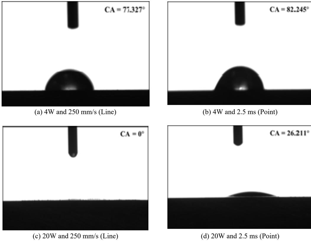
**Figure 4** Water droplet on laser-textured surface produced by using the different processing conditions
