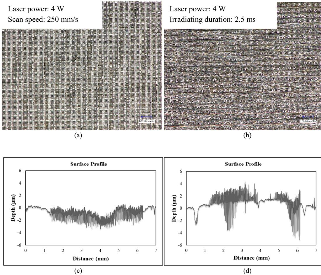
Figure 2 Surface morphology and profile of AISI 316L stainless steel after (a, c) line and (b, d) point texturing
