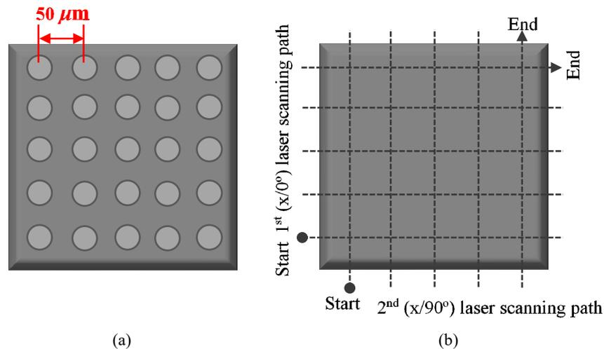
**Figure 1** Laser texturing patterns applied in this study: (a) point; (b) line
