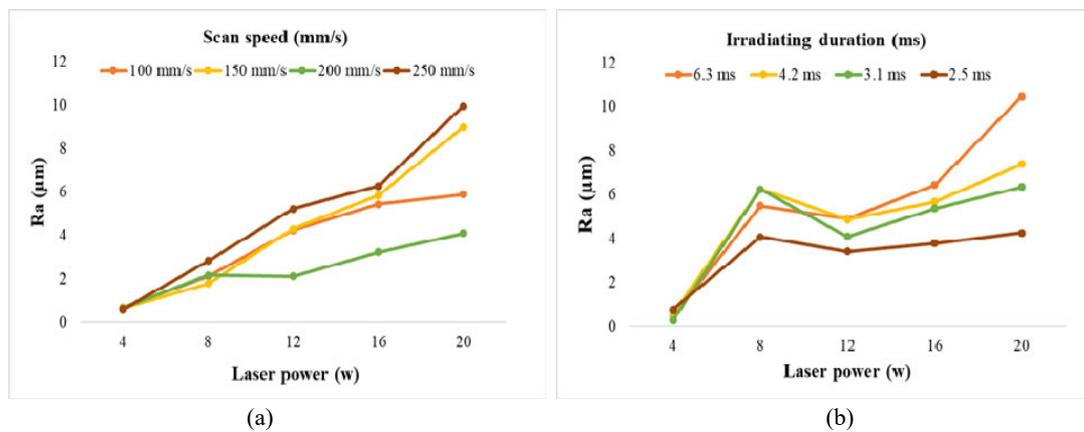
Figure 3 Effect of laser power and scan speed on surface roughness when texturing the (a) line and (b) point patterns
