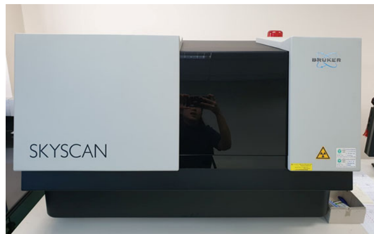
Figure 1 Micro-CT object scanner (Skyscanner 1173, Bruker Company, Belgium)
