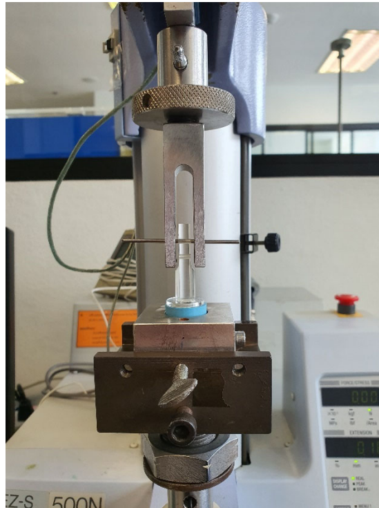
Figure 2 Sample placed for tensile bond strength test in a universal testing machine
