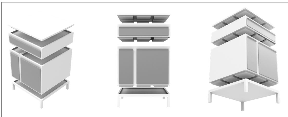
Figure 3 Exploded view of an add-on module joining system.
