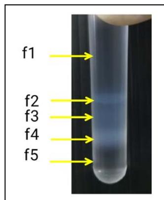
**Figure 5** Separation of intracellular proteins obtained from recombinant VP2 baculovirus-infected Sf9 cells in 25-70% sucrose gradients after ultracentrifugation at 33,200 rpm for 90 min at 4°C
