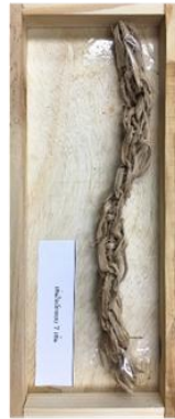
Figure 9 Knitting rope seven lines when load water 9 liters pattern tissue start torn off and tear, when weighted 11 liters.
