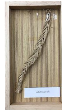
Figure 10 Knitting rope eight lines when load water 7 liters pattern tissue start torn off and tear, when weighted 9 liters.
