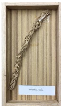
Figure 7 Knitting rope five lines when load water 6 liters pattern tissue start torn off.
