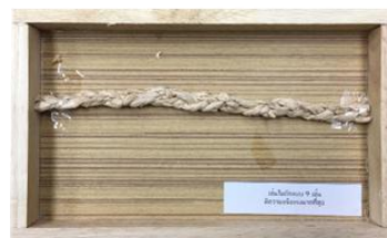
Figure 11 Knitting rope nine lines when load water 15 liters pattern tissue start torn off and tear, when weighted 17 liters.
