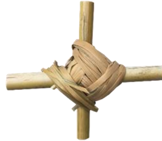
Figure 15 The outer surface of the weave pattern 4. Connection by rope. Which provides a connection strength and was moving slightly.
