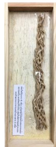
Figure 8 Knitting rope six lines when load water 5 liters pattern tissue start torn off and tear, when weighted 7 liters.
