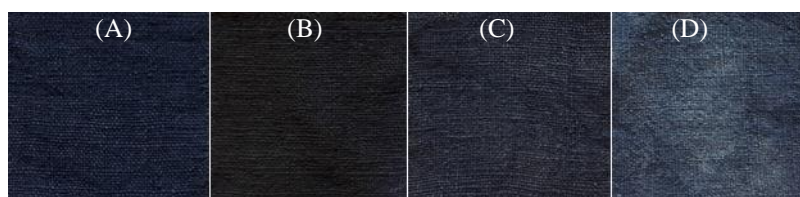
Figure 2 The cotton fabric dyeing using Indigo and various mordants ; Indigo and water (A), Indigo and Nypa palm (B), Indigo and mud (C), Indigo and fly ash (D)
