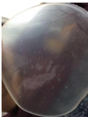
Figure 5 The mcl-PHAs biopolymers film prepared by casting the PHA-chloroform solution onto a Petri dish and allowing the solvent to evaporate at room temperature for 1 week
