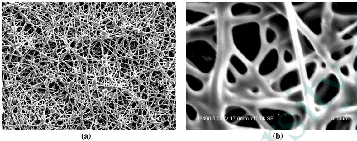
**Figure 2** SEM images PHA/DCM electrospun nanofibers 8%PHA/DCM at 1,000x (a) and 10,000x (b) magnification
