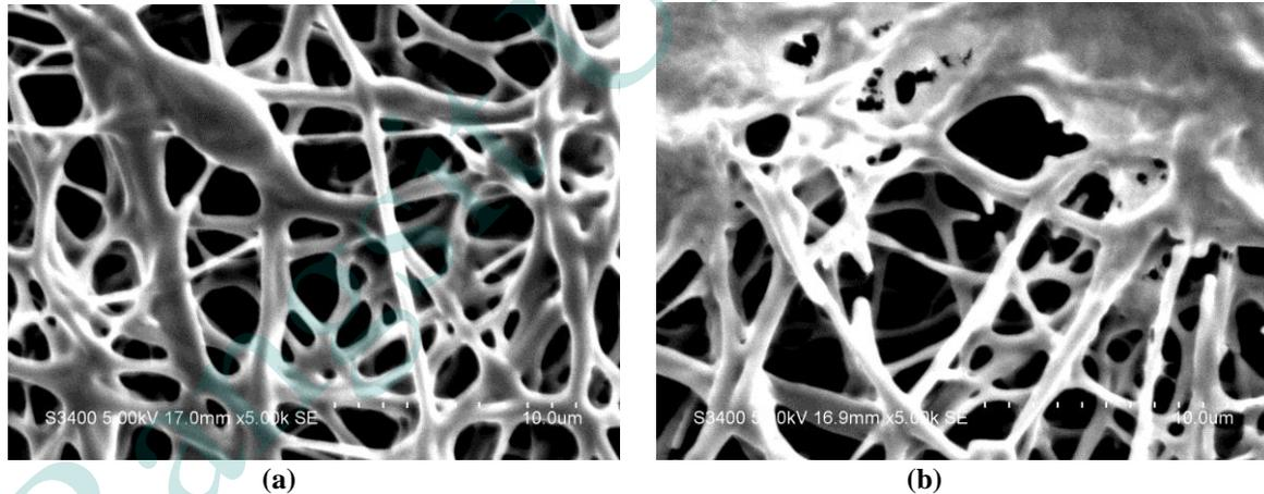
**Figure 3** SEM image of PHA/DCM electrospun nanofibers 8%PHA/DCM at 5000x (a) and SEM micrograph of HaCaT cells on the electrospun PHA nanofiber in magnification of 5000x (b)
