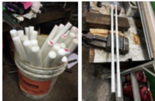
Figure 3 and 4 POM materials (polyoxymethylene)
