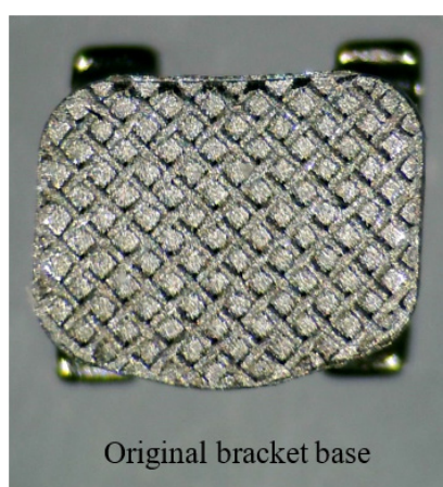
Figure 2 Illustration from stereomicroscope image of bracket base before bonding, showing surface condition for ARI comparison.
