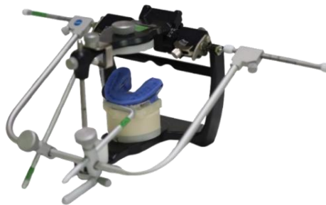
Figure 2 The customized transfer tool was positioned on the lower member of the MA
