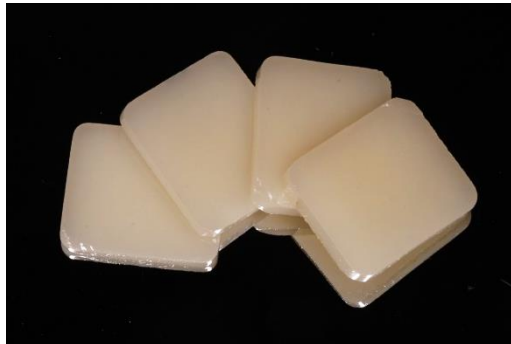
Figure 3 Specimens were sectioned from E.max CAD blocks in four thickness
