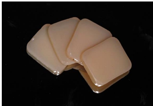
Figure 4 Specimens were sectioned from CEREC Tessera blocks in four thickness
