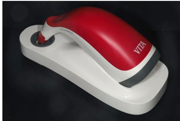
Figure 5 The spectrophotometer (Vita Easyshade) and its charging station
