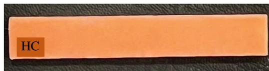
**Figure 4a** Polished unreinforced heat-polymerized acrylic resin specimen (65x10x3 mm<sup>3</sup>)
