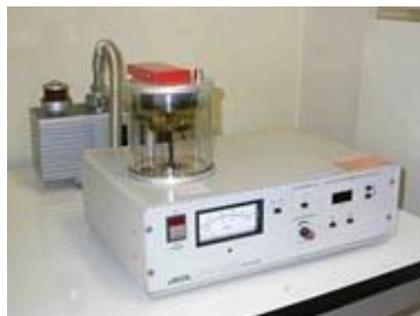
**Figure 6** Gold Coater Jeol Model JFC-1200
