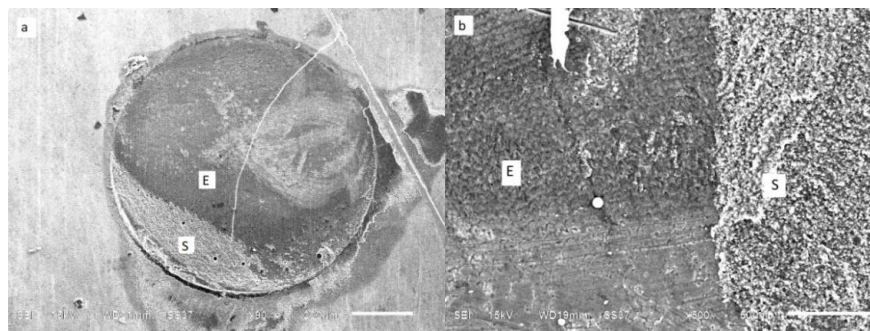
Figure 6 SEM photomicrography illustrating mixed failure for UltraSeal XT™hydro™ sealant at 90x (a) and 500x (b) magnifications; (E-etched enamel surface; S-sealant)
