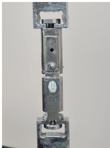
Figure 3 Shear force produced by orthodontic wire around the bonded specimen.
