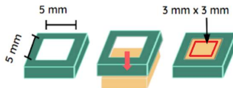
Figure 2 shows the pattern of a putty index to assist in selectively locating the area of the testing site.
