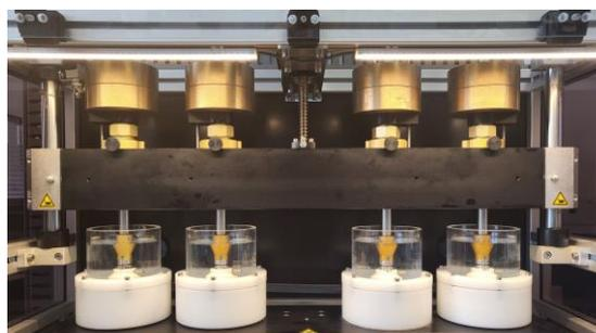
**Figure 2** The specimens and their antagonists were mounted in a chewing simulator
